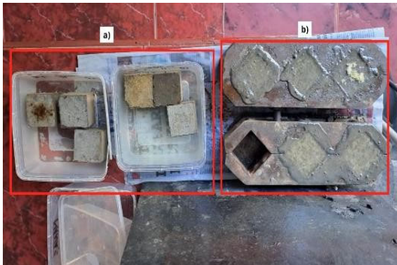
Figure 2. Mortar cube specimens: (a) water curing, (b) fresh mortar in molds.
