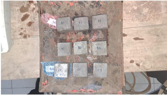
Figure 3. Mortar cube specimens (50 × 50 × 50 mm) of non-control mixtures incorporating natural fibers, labeled and prepared for compressive strength testing.
