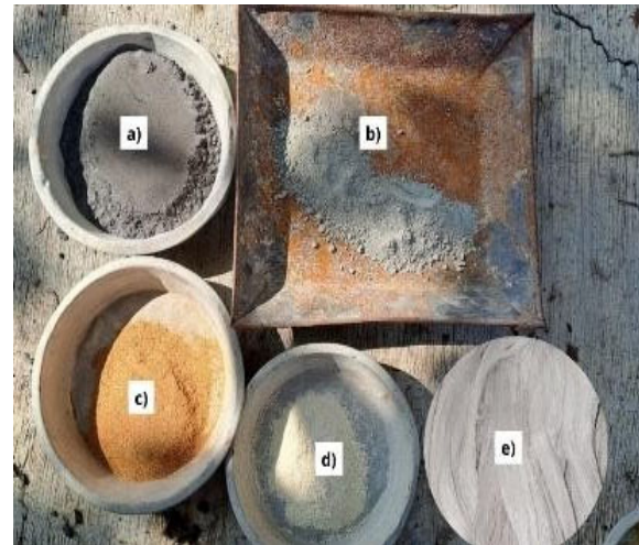
Figure 1. Raw materials used in the mortar mix: (a) tabas sand, (b) portland cement, (c) CCF, (d) BF, and (e) PLF
