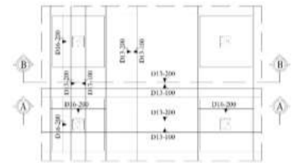
Figure 3. Reinforcement Plan for Flat Slab and Drop Panel on Floor 4 th floor
