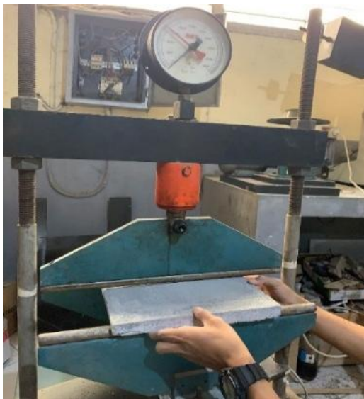
Figure 3. Flexural strength test for concrete roof tile samples.
