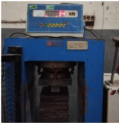
Figure 2. Compressive strength test for mortar samples.
