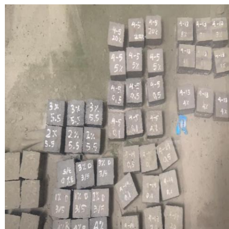
Figure 1. Cubic-shaped mortar samples after curing process.
