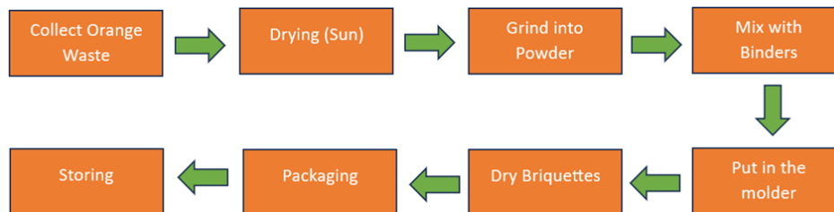
Figure 8. Flowchart on making orange briquettes
