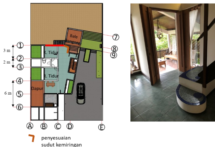
Figure 4. Ground floor plan of the second house with adjustment of the walls to the slope angle of the bale bengong structural module, and adjustment of the stairs to the circulation space.
