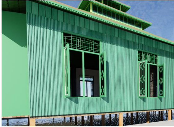
Figure 9. Proposed full-height louver window design Source: Fitriyanto, et.al, 2025
